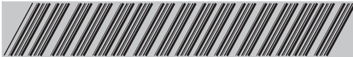
Helical scan tape format
